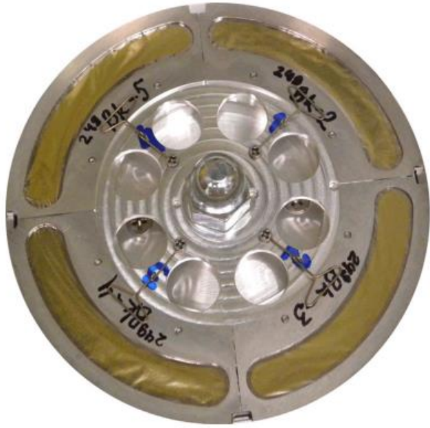
Figure 13: Assembled TASCA target wheel with four target segments, containing a total amount of about 12 mg ^{249}\text{Bk} , deposited by molecular plating on 2\ \mu\text{m} Ti backings [144]. The total ^{249}\text{Bk} \beta^- activity was 6 \cdot 10^{11} Bq at the beginning of irradiation [86]. (Reprinted by permission from Springer nature Customer Service Centre GmbH: Nature Springer J. Radioanal. Nucl. Chem. 299, 1081–1804 (2014), “Preparation of actinide targets for the synthesis of the heaviest elements”, https://doi.org/10.1007/s10967-013-2616-6 , J. Runke et al., © 2014).
