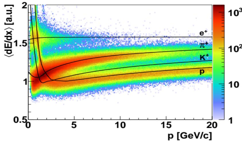
$$\left\langle -\frac{dE}{dx} \right\rangle = K z^2 \frac{Z}{A} \frac{1}{\beta^2} \left[ \frac{1}{2} \ln \left( \frac{2m_e c^2 \beta^2 \gamma^2 W_{max}}{I^2} \right) - \beta^2 - \frac{\delta(\beta\gamma)}{2} \right]$$
