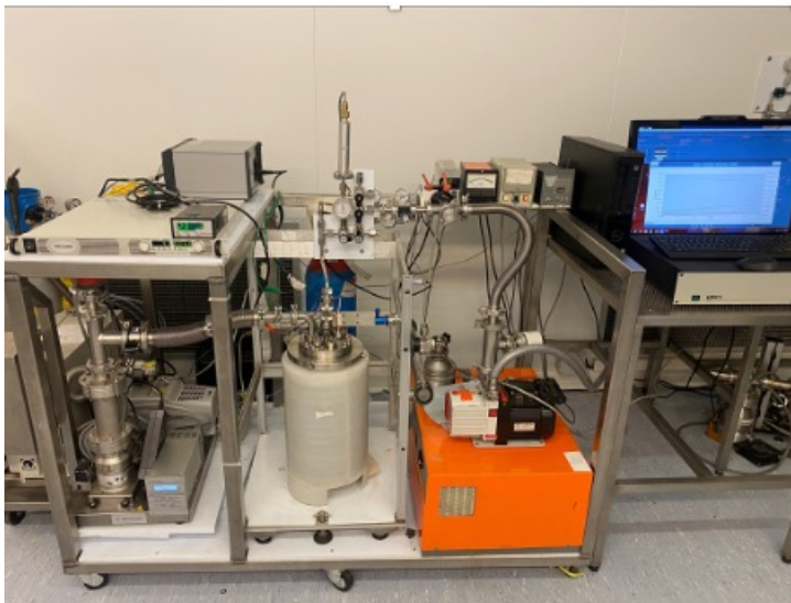
Large Quartz cell able to contain up to 1kg of powder
