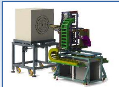
BEta-deLayEd Neutron detector ( BELEN ) 48 3 He cylindrical counters
