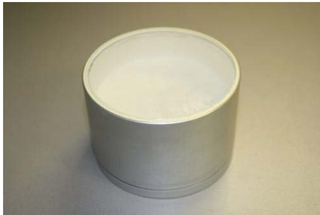
Stilbene crystal: \varnothing 80 mm, thickness 50 mm
