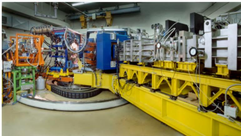
PRISMA Magnetic spectrometer
